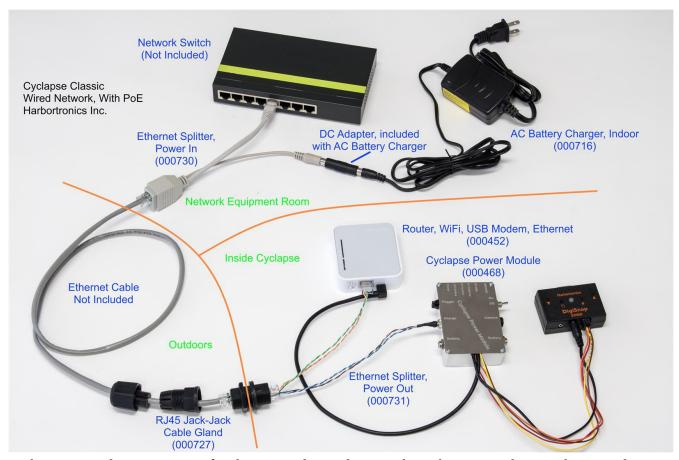
In this picture, the connections for the optional Wired Network, with PoE are shown. There are three 'locations' shown, the Network Equipment Room, the inside of the Cyclapse housing, and the Outdoors. It looks complicated, but if you follow the picture, it should be very easy to install.
