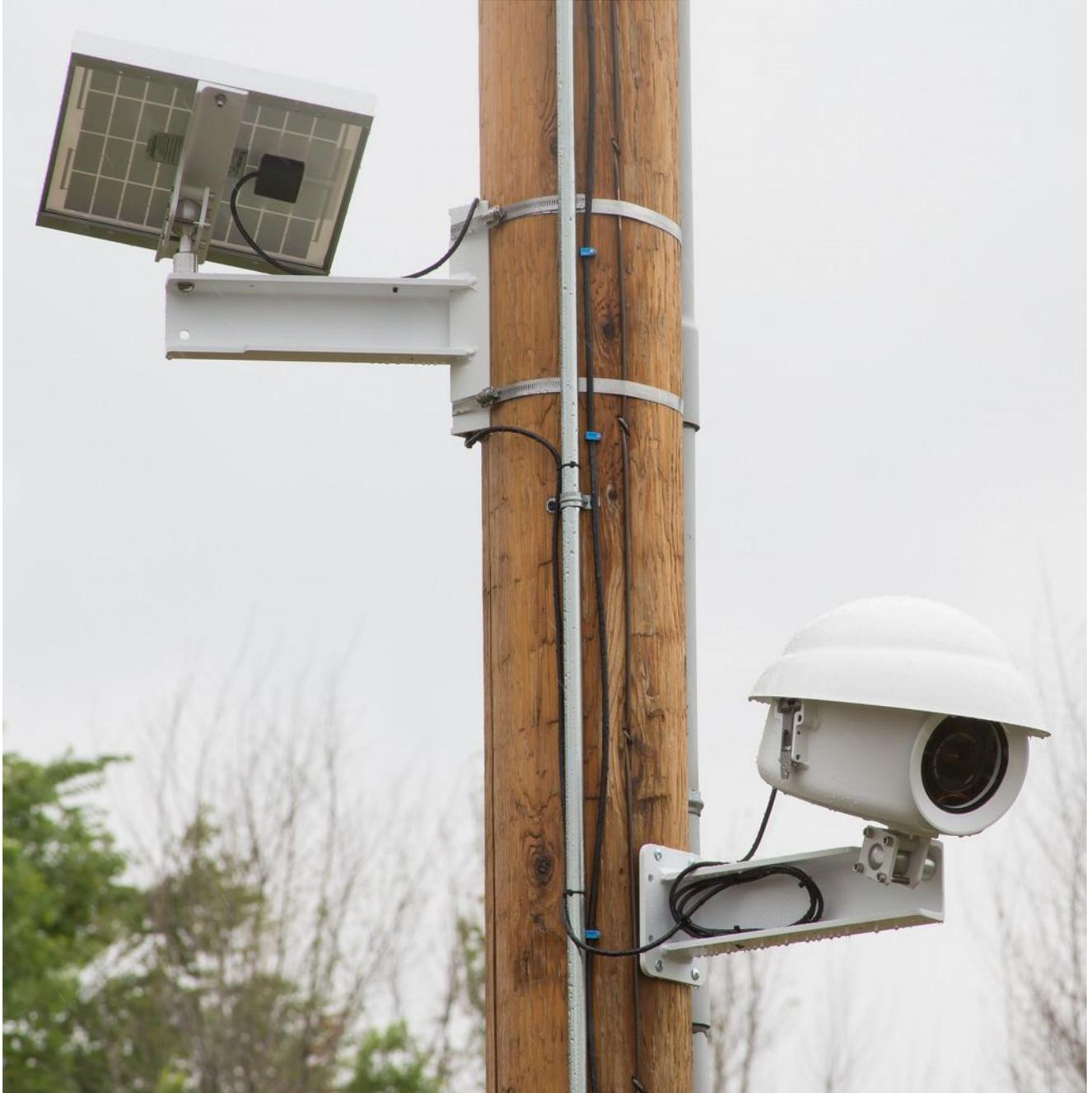
**Cyclapse system, illustrating the two mount arms, operating on a utility pole in the rain.**
