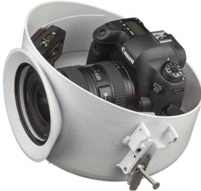
**Canon 6D camera in housing, with 16-35mm lens (lid removed)**
