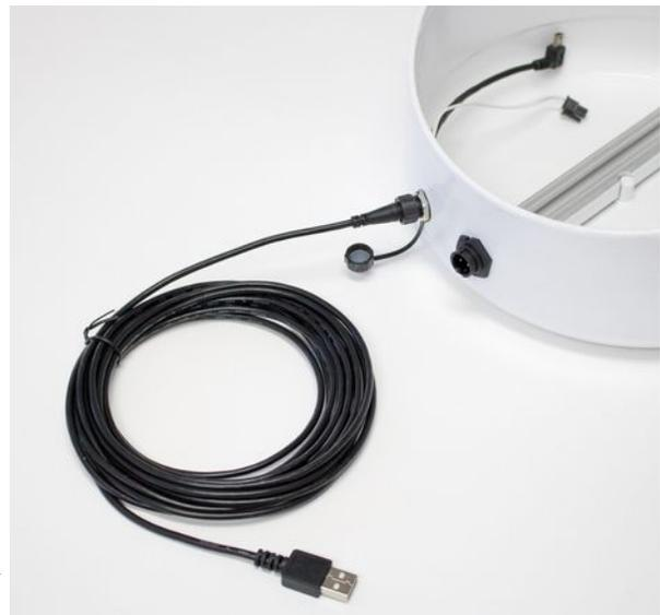
The cable can be removed if not using the USB extension option, but please cap the connector to maintain the seal on the housing!
