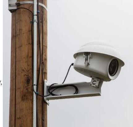
The window is sealed and is made from borosilicate glass, using anti-reflective coating on the inside to reduce interior light reflections into the lens. The outside surface of the window is not coated, preventing any optical issue with gradual coating erosion in the elements or concerns for cleaning.
